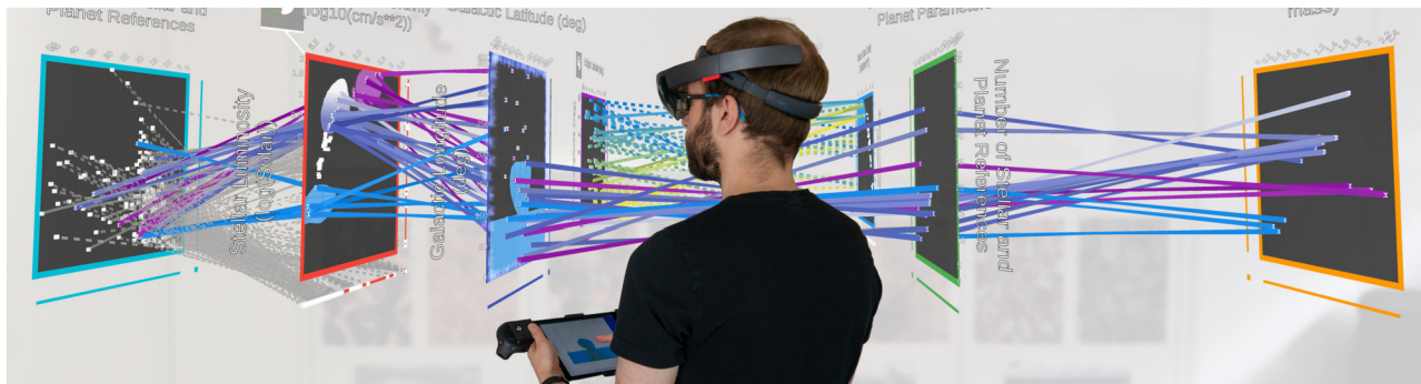
Figure 1: STREAM combines spatially-aware tablets with augmented reality head-mounted displays for visual data analysis. Users can interact with 3D visualizations through a multimodal interaction concept, allowing for fluid interaction with the visualizations. [9].
