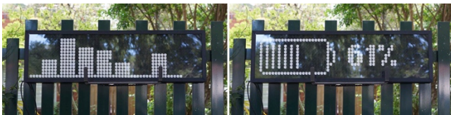
Figure 3. Exploration of various visualizations of energy usage [33]: weekly graph (left), battery pictogram (right).
