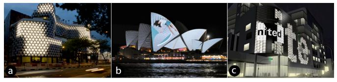
Figure 1: Examples of different media façade types in different locations: (a) Low-resolution light emitting façade type, (b) frontprojection high-resolution type and (c) high-resolution screen embedded in a low-resolution light emitting façade. Image credits: (a) and (b): © realities:united, (c): © Jerry Dohnal.
