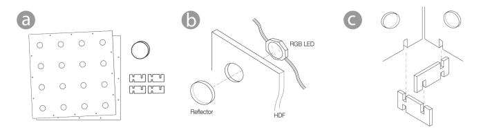
Figure 2: Construction manual for hybrid media façade toolkit: (a) laser cutted wooden façade panels, acrylic reflectors and joints for assembling (b) attaching the reflectors ahead (gluing is recommended) and inserting the RGB-LED chains from back (c) assembling the modular panels with the joints.
