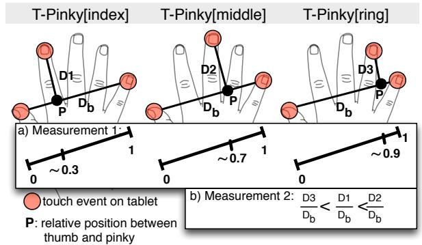
**Figure 4.** Thumb-Pinky basis family (T-Pinky): a) index, middle and ring finger are at a common relative position between thumb and pinky. b) relative distances between basis fingers and third finger are different.
