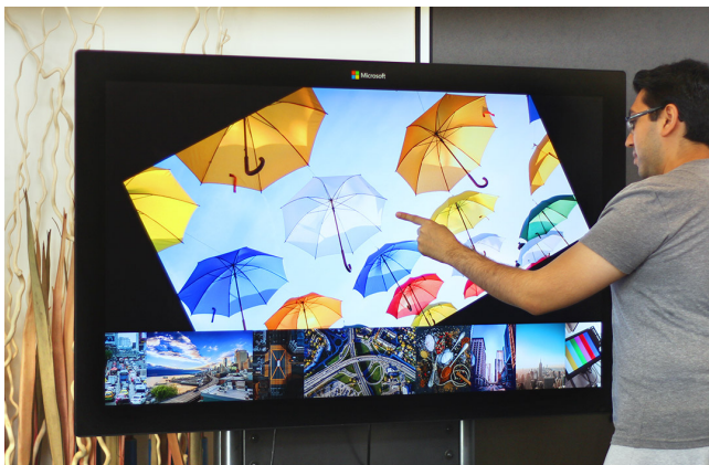
Figure 4: For images or maps, pitch and yaw can be used to rotate and zoom the object. We present a mock-up to demonstrate how rotate and zoom works in a gallery on a wall-sized display.
