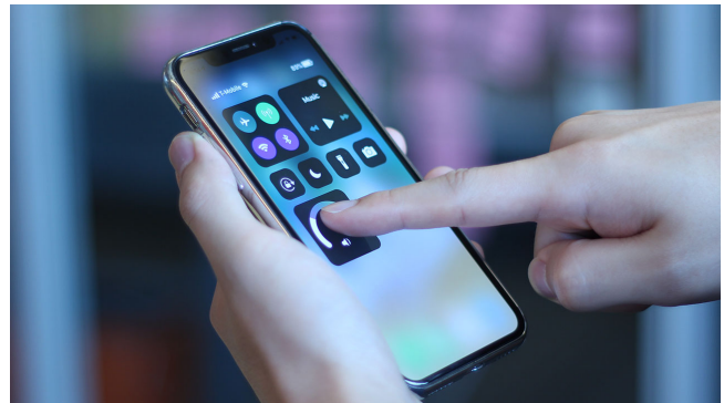
Figure 1: A mock-up implementation of a circular slider which can be controlled with the finger's yaw. As depicted in this image the users finger controllers the volume using a circular slider.
