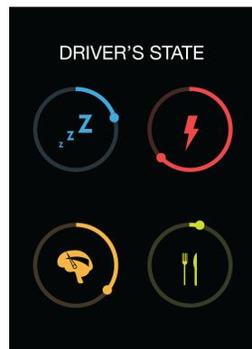
**Figure 2:** The *dashboard* continuously displays all four states to the driver. Each state is visualized by an icon and a circular progression indicator.
