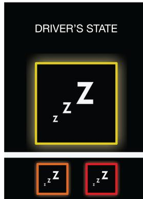
**Figure 1:** An *on-time warning* is displayed when a critical value is reached (here: drowsiness). A warning features a color-coded frame indicating the urgency.
