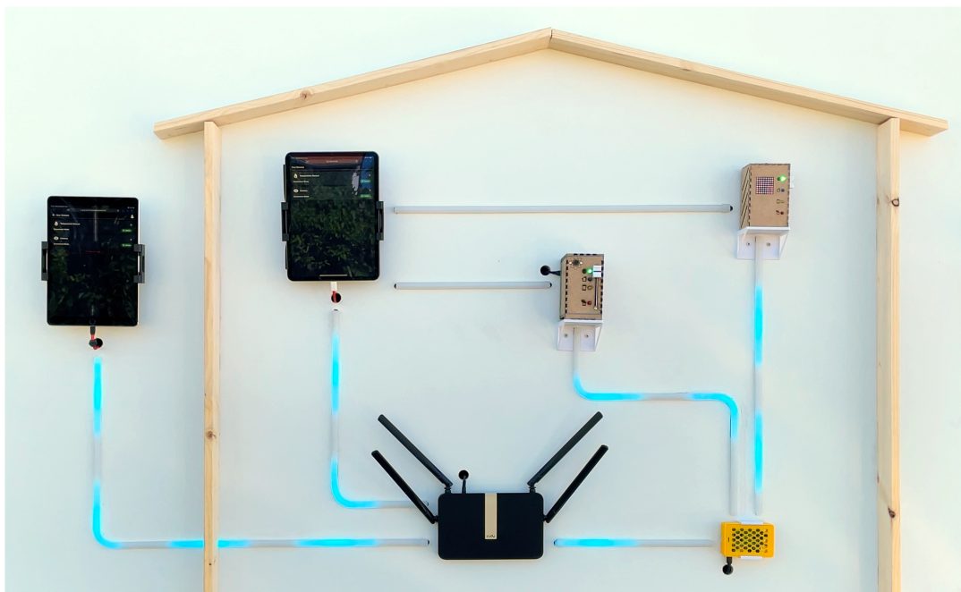
Figure 1: Ecosystem Demonstration of Connectivity Control visualizing the data flow between two smart devices, a hub, a router, and two tablets
