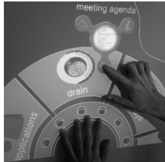
Fig. 5. The two hands cooperate in manipulating information: the dominant one drags a unit of information on the drain to delete it.
