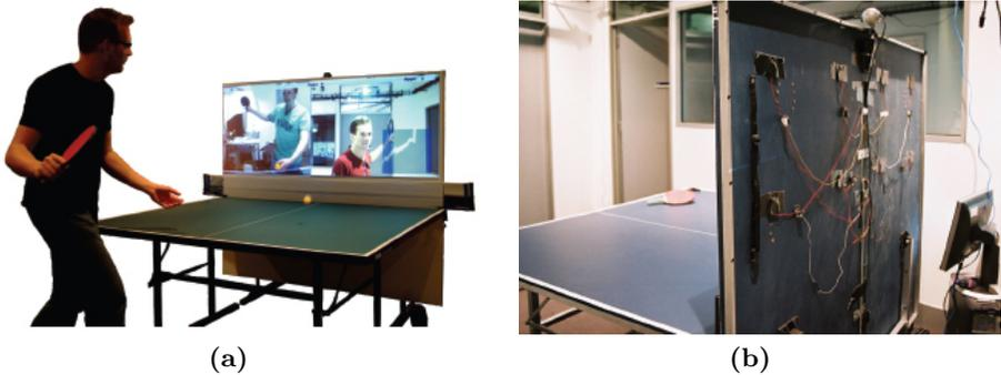
**Fig. 5.** "Table Tennis for Three" (Mueller and Gibbs, 2007). (a) Table with video conference projection, (b) impact detection mechanism.
