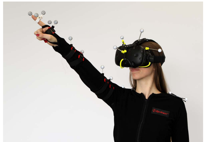
Figure 1. User with the marker set of rigid bodies for finger, forearm, upper arm, head, left, right shoulder, and head (HMD).
