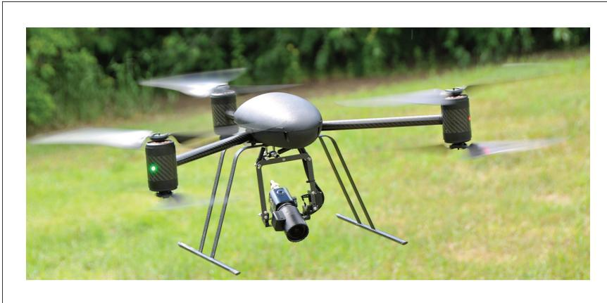
Figure 2. Camera mounted to a Draganflyer X6 drone. (Photo courtesy of DraganFly; [www.draganfly.com](http://www.draganfly.com).)
