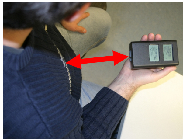
Figure 1. A user interacting with the DistScroll. By moving device as the arrow indicates, he scrolls through the menu entries of a fictive application depicted on the top display. On the bottom display additional state information is presented.
