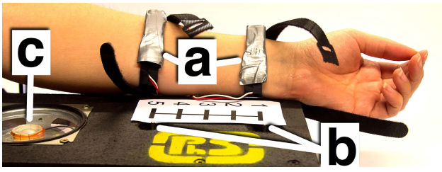
Figure 2: We compared three actuator technologies in a user study: (a) Eccentric vibrational motors (integrated in an elastic arm sleeve) (b) solenoids (c) voice coil actuators
