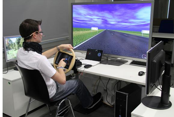
Figure 1: The study setup with multitouch steering wheel and speech input in the simulator.
