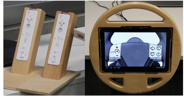
**Figure 7: Controls used to approximate a traditional automotive interface.**
