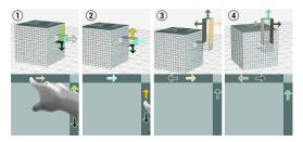
Figure 2. Extrusion workflow: arrows in the diagram indicate perspective-dependent polygon selections and the according gestures on the extrusion touch pad. (3) and (4): polygon selections flip when the view is rotated.
