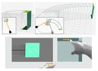
Figure 3. Creating bent shapes with simultaneous extrusion and camera control.  $\alpha$  is the angle of camera rotation and corresponds to the sum of rotation angles of the automatically extruded polygons.
