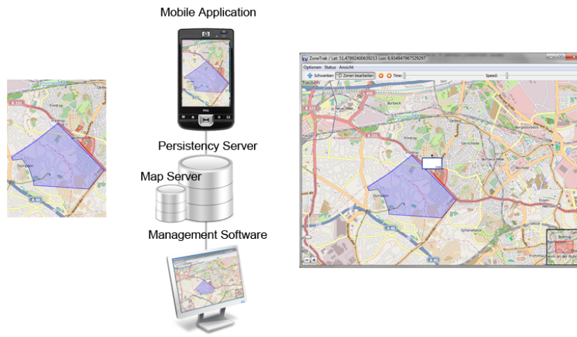
Fig. 1. ZoneTrak architecture scheme
