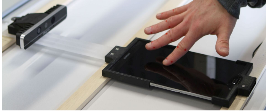
Figure 1: The prototype with the 8.4-inch tablet and the depth camera.
