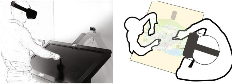
**Fig. 2.** Left: An HMD user acting in the virtual world with haptic feedback. Right: A short term interaction between a RW user and a HMD user with a shared frame of reference by using a mobile projector with touch recognition.
