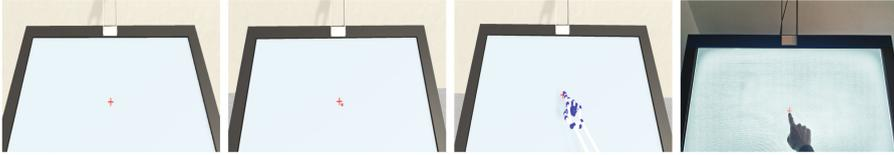
**Fig. 1.** Conditions during the haptical supported pointing task from left to right: No Feedback (NO\_FB), rendering the touched position (TOUCHPOINT\_FB), continuous visual feedback of the hand provided by handtracking (HAND\_FB) and the real world baseline (RW\_BASELINE)
