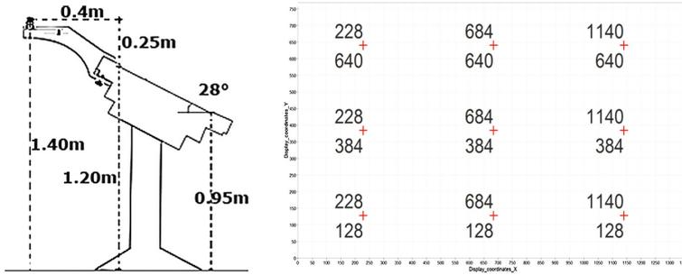
**Fig. 3.** Drawing of touch table dimensions (left) and the target positions in pixel coordinates on the screen (right). (Color figure online)
