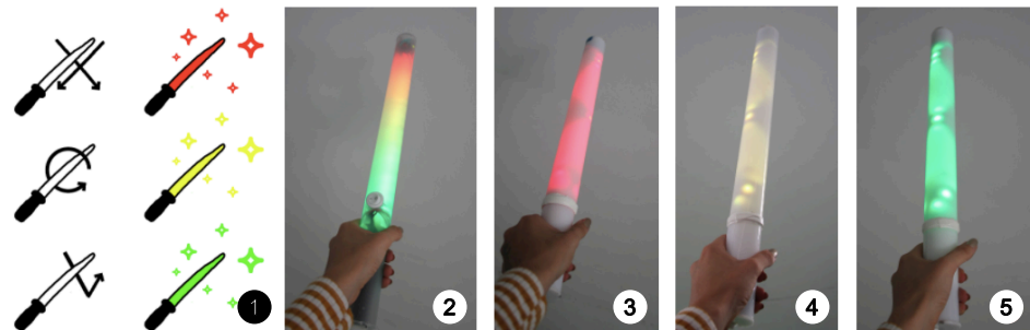
Figure 6. Glowing Wand technical prototype (1. different hand gesture designs; 2. switch for a rainbow feedback; 3. negative tick gesture to red light; 4. circle gesture to yellow light; 5. tick gesture to green light).
