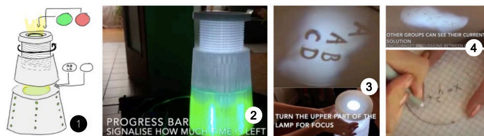
Figure 3. stayFOCUSed technical prototype (1. concept idea and structure; 2. show timer with light progress bar; 3. rotate the lamp to show answers; 4. pen-writing on the disk).
