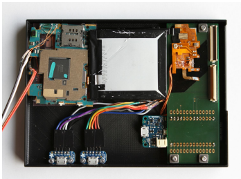
Figure 4: The Hardware Container containing the PCB that is connected to the circuit board and batteries of two Nexus 5, and an Arduino to operate the capacitive side sensors.
