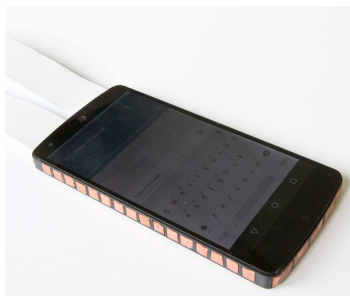
Figure 2: The Touch Device with a front and back touchscreen, and capacitive sensors on the sides.
