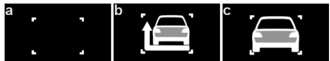
Figure 1: Displaying a rectangular marker, even when no warning is active (a), can provide visual reference and may improve perception. Two different warnings indicate a different reaction (b: evade , c: brake ).
