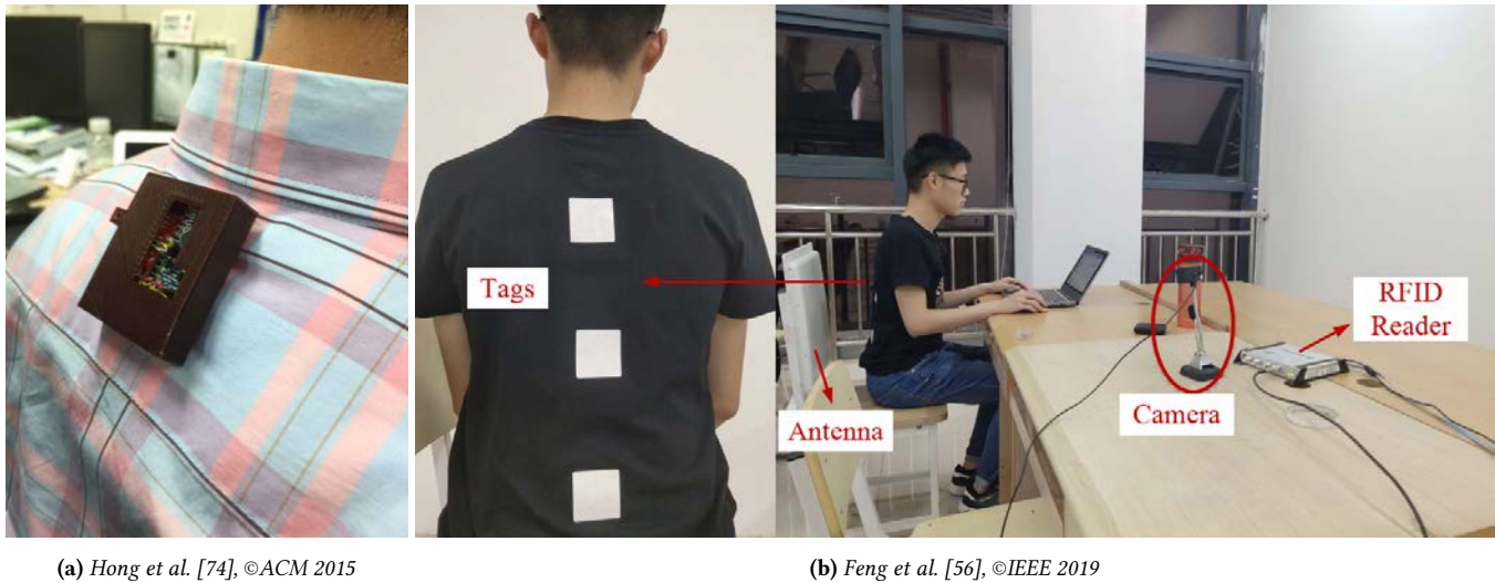
Figure 3: Examples of motion and distance sensors for sitting posture recognition: (a) a gyroscope attached to the upper back and RFID tags on the lower, middle, and (b) upper back with the corresponding antenna attached to the backrest of a chair
