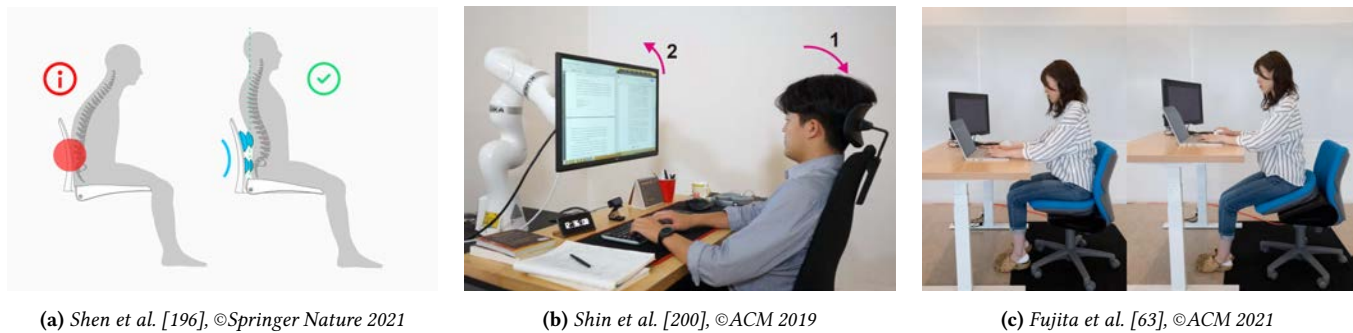
Figure 7: Examples of actively correcting the user's sitting posture: inflatable bladders on a chair (a), a self-adjusting computer display that can be tilted (b), and the combination of a self-adjusting chair that can be inclined and a sit-stand desk (c).
