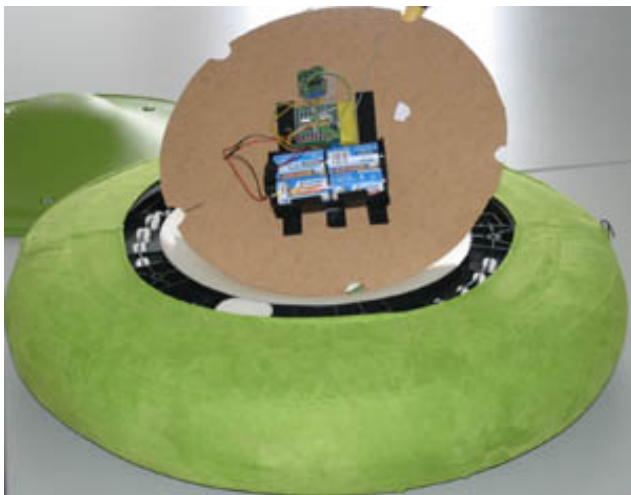
Figure 4: Opened Virrig with the integrated Smart-Its.
