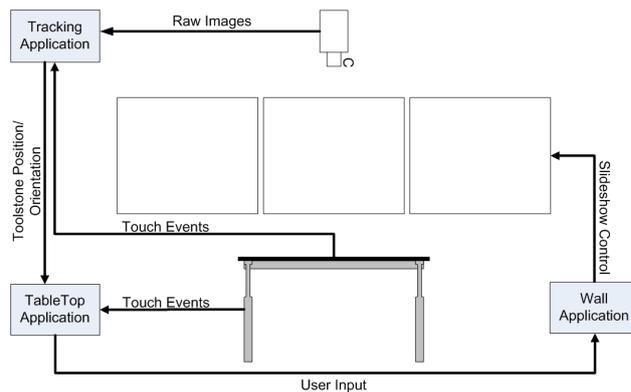
Figure 2: Architecture Overview of the Living-Room prototype.
