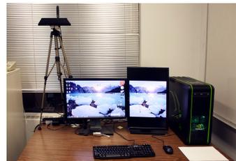
**Fig. 3.** The *Unadorned Desk*: a Kinect tracks the user's hand
