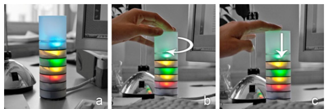
Figure 1. StaTube is a tangible presence indicator located on the user's desk: Each ring represents a Skype contact with the top-most ring as one's own state (a). Rotating allows for changing one's own state (b). Pressing the tube sets a timer for when a user will return to the desk (c).
