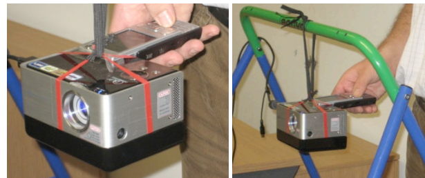
Figure 1. N95 attached to the handheld projector to simulate real use in the experiment.
