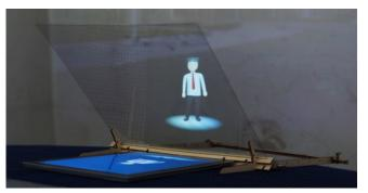
Figure 4. The head-up display was designed to not interfere with the participants' view of the road scene and shows a clear and bright image.
