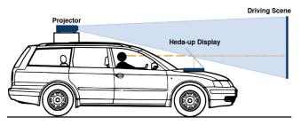
Figure 3. The projector was placed on the roof of a Volkswagen Passat so that the projected image covered the entire field of regard through the windshield.
