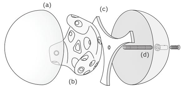
Figure 2: The spherical controller is constructed from a two-piece acrylic glass sphere with a diameter of 12 cm (a) that encloses a Vive Tracker (b). A stabilization piece (c) centers and stabilizes a 1/4 inch threaded rod that is screwed to the sphere from the outside (d).
