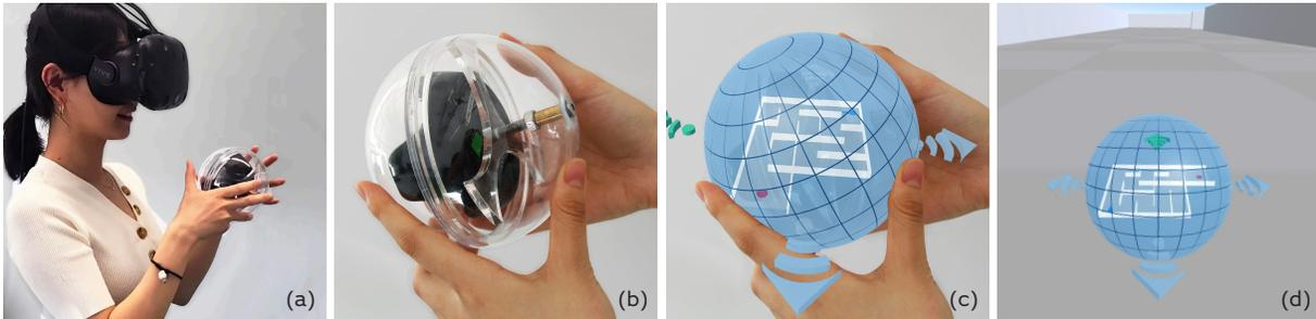
Figure 1: We show how a handheld (a), tracked spherical object (b) aligned with a visualization (c) can be used to control first-person locomotion (d) in virtual reality (VR) by means of rotation. We implement two different approaches (*Position Control*, *Velocity Control*) and compare them to two established methods using VR controllers. Our results show that the spherical controller in combination with the position control technique leads to both faster task completion and higher accuracy.
