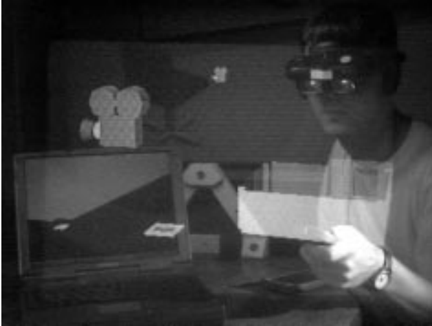
Figure 2. An EMMIE user manipulates a 3D model with an optically tracked hand-held pointer. Other virtual objects shown include simple iconic 3D representations of applications (e.g., a “movie projector” that can play videos) and data objects (e.g., “slides” that represent still images).
