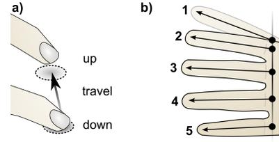
**Figure 4.** A touch event (a) and the hand model (b) with lines indicating slopes and intercepts along the touch surface edge on the back. The index finger is modelled with two lines to account for the abducted stance used to reach the second row of keys (compare to Figure 2).
