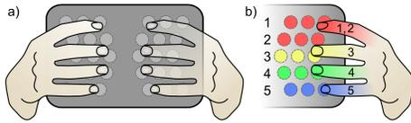
**Figure 2.** A folded multitouch keyboard [28] on the back (a) with finger-to-key assignments (b). Each key is associated with one character, depending on the layout (e.g. QWERTY). Keys in this figure are not personalised; our approach adapts locations and sizes of keys to the user.
