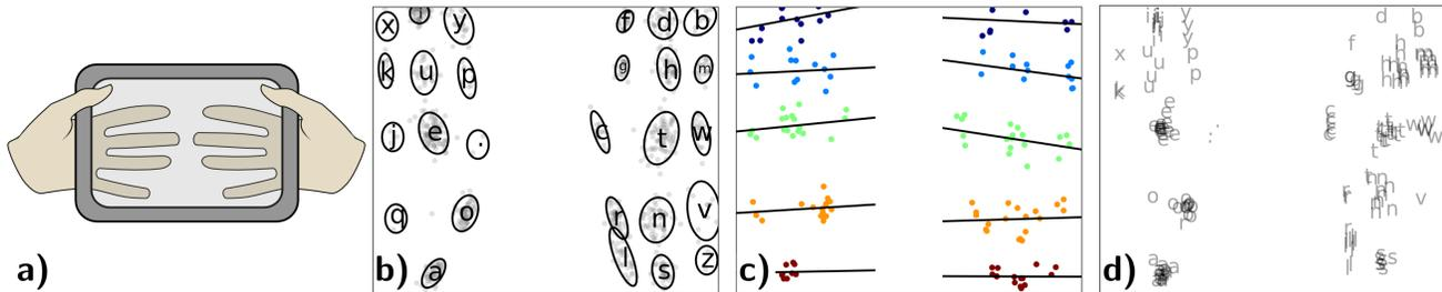
Figure 1. We present a method for ten-finger typing on the back of a tablet with a capacitive multitouch sensor (a). b) Gaussian Bayes learns keys from labelled touches and c) hand modelling assigns *new* unlabelled touches to fingers, represented as lines. Both models are combined in a clustering method to predict characters for touches (d) and adapt keys when hand postures change during typing. We further improve predictions with language models.
