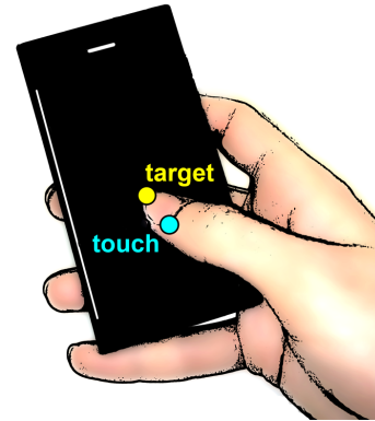
Figure 1. Touch offset. The user intended to hit a target to the upper left of the actual touch location. The difference between both locations is a two-dimensional offset vector. Given previously recorded touch data, offset models can predict the target location for future touches to improve the user's touch accuracy.
