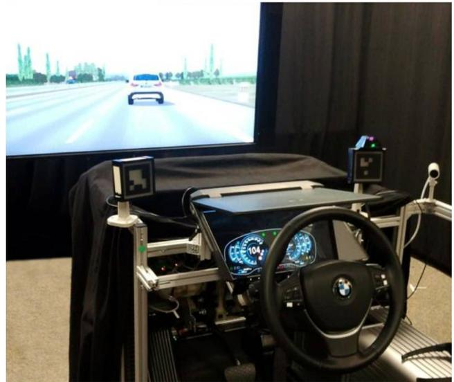
**Figure 1:** Setup of our experiment: We use a driving simulator to evaluate the influence of visualization, technology, and interface complexity on user performance and subjective perception of S3D user interfaces.
