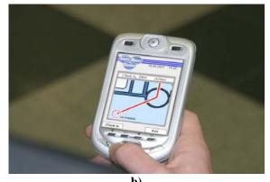
Figure 2: An MEM providing details about a flight (a) and showing the way to the next check-in terminal (b)
