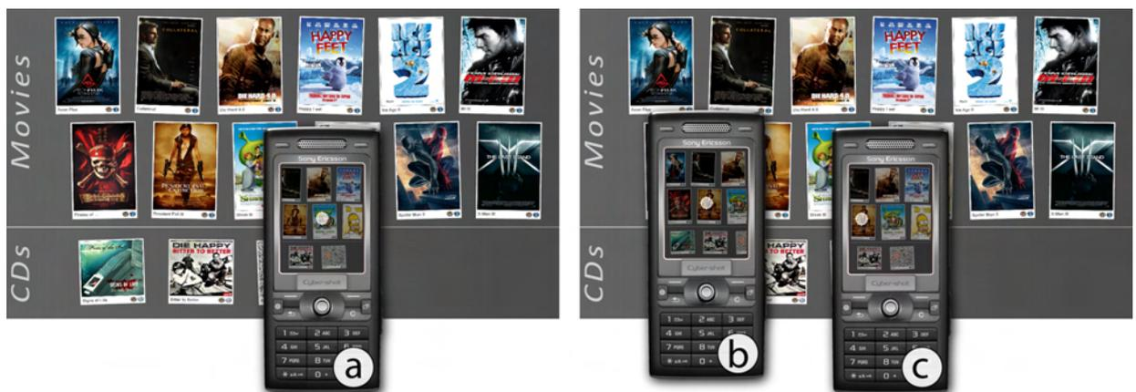
**Figure 5.11:** Comparison of moving the device versus moving the crosshair: the user aims at a movie (a) and wants to select another. The user has to either move the device to get the new content underneath the crosshair (b) or shift the crosshair to the desired content (c).
