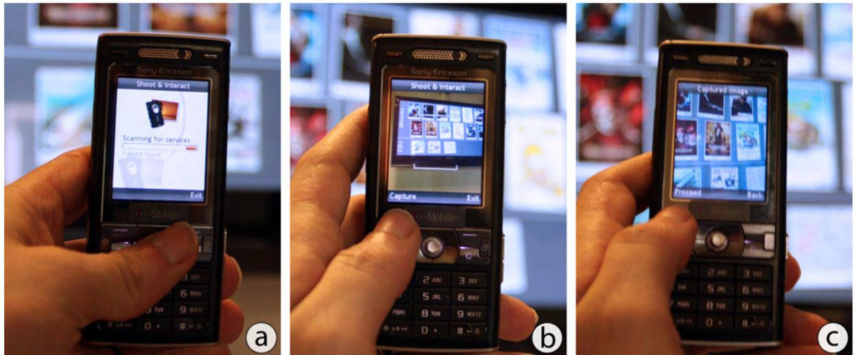
**Figure 5.7:** Connecting and selecting content *through the display*: While the application launches, the system connects to the display already with a specialized service name (a). Then the camera preview is shown which allows users to aim at content of interest (b). After capturing an image, users can decide whether this image has the content in its center (c).
