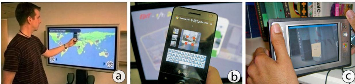
**Figure 2.15:** Virtual content shown in live video on mobile devices: a) The device's position and orientation is used to interact with content (through markers) [MSSU04]. b) Dynamic markers are used to obtain the transformation between mobile device and remote display in 3D [PJO09]. c) The *iCam* allows to place content at three-dimensional positions [PRA06].
