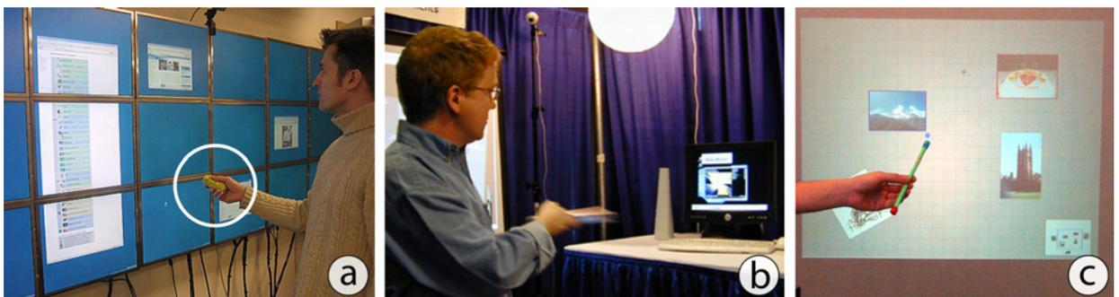
**Figure 2.7:** Controlling a pointer on distant displays: a) *Soap* controls a mouse pointer in mid-air [BSW06]. b) The *XWand* can be used to point at distant screens further allowing gestures to control the content [WS03]. c) *VisionWand* uses two cameras to detect both ends of the wand to obtain its position and orientation [CB03].
