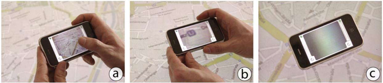
**Figure 8.6:** Problems of live video with directly superimposed displays: (a) At distances of several inches users can interact in a sharp video image. (b) Getting closer blurs the video image. (c) Placing the camera on the external screen makes the video unusable.
