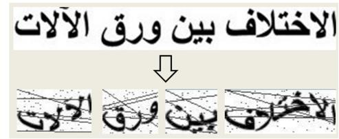
Fig. 2. Adding random waves, dots and lines as extra degradations to cropped images
