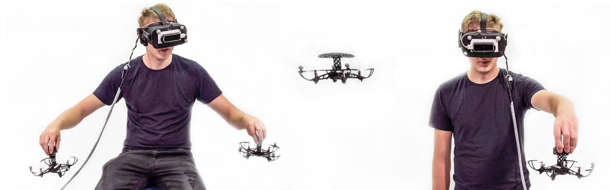
Figure 1: Left: A user piloting an aircraft in VR. The user has a slider in his right hand to control the speed. With the joystick in his left hand, the aircraft can be steered sideways. Right: A user is rotating an object in VR using a knob.
