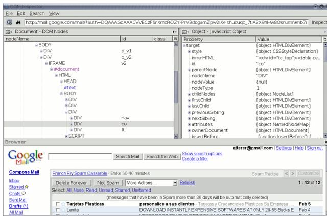
**Figure 2: The Firefox DOM inspector tool allows the user to browse through an AJAX application’s DOM tree (top-left part of the window) in real time.**
