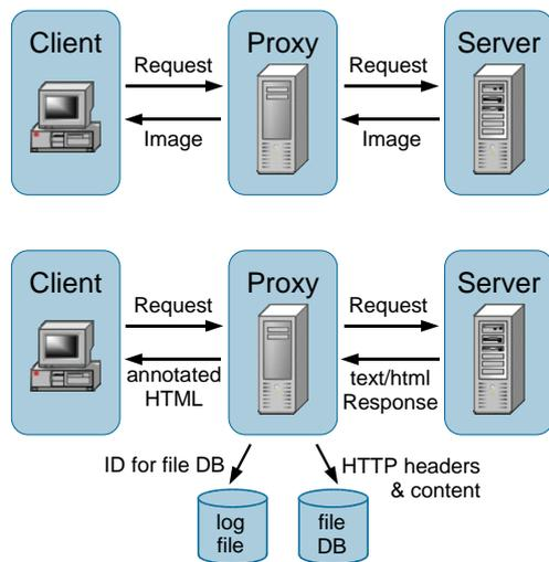
**Figure 1: UsaProxy passes on images and other data unmodified (top). HTML content is modified (bottom) by adding special JavaScript. Also, the server response is recorded and identified via a logged ID.**
