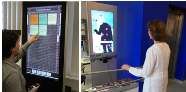
Figure 1: Examples of interactive applications in public spaces with direct touch based (left) and indirect gesture based (right) interaction. For more examples see [2].
