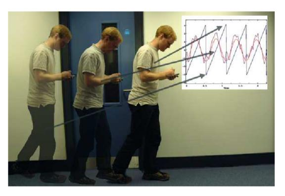
Figure 2. A user walking with the device and corresponding acceleration trace. The unfiltered vertical acceleration signal (rough sinusoid), the filtered signal (smooth sinusoid) and the phase estimate (in radians) for the signal (saw-tooth).
