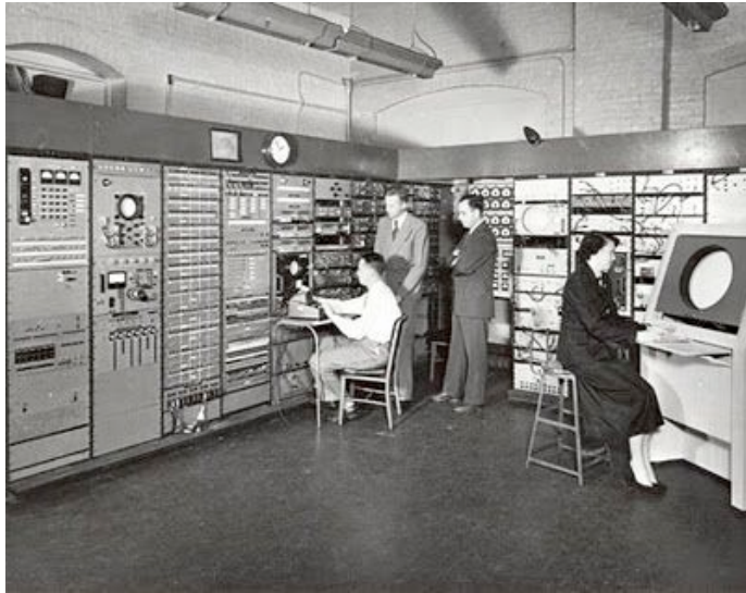
1945-1952: "Whirlwind" computer (Jay Forrester, MIT) Digital computer using oscilloscope screen displaying real-time aircraft data, later "SAGE" system
