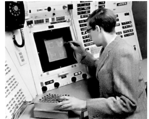
1957-1969: "TX-2" computer at MIT Lincoln Lab Transistor-based computer providing interactive graphic displays L.G. Roberts, 1962: 3D Graphics Ivan Sutherland, 1963: Sketchpad
