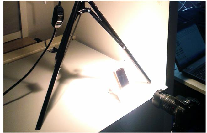
Figure 7. To perform smudge attacks, an HTC Nexus One was placed under an Arri 650W spot light and in front of a Canon EOS 1000D. Under such overexposed conditions, even minor residues become visible.
