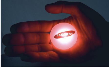
**Figure 1.** The physical interface from *SoloFind* as experience prototype, equipped with a hi-power light emitting (LED) diode and a Near Field Communication (NFC) tag.
