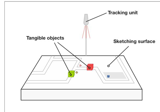
**Figure 6:** The conceptual drawing: A rewritable surface on which self-propelled tangible objects move, controlled by a tracking module mounted in a tripod.
