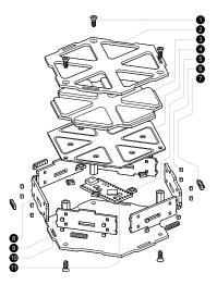
Figure 9. (1) screws, (2) top, (3) silicone-pad, (4) PCB, (5) WS2812b LEDs, (6) magnets, (7) spring loaded connectors, (8) flanks, (9) bottom, (10) spacer, (11) Teensy LC.
