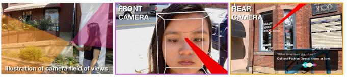
Figure 1. WorldGaze simultaneously opens the front and rear camera on smartphones. The front camera is used to track the user's 3D head vector, which is then raycast into the world as seen by the rear camera. This allows users to intuitively define an object or region of interest using their head gaze, which voice assistants can utilize for more precise and natural interactions (right bottom).
