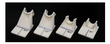
Figure 3. The four pitch stabilizers we used in the study to limit PITCH to  $77.5^{\circ}$ ,  $55^{\circ}$ ,  $32.5^{\circ}$  and  $10^{\circ}$  presented from left to right.
