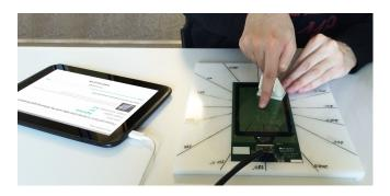
Figure 4. The apparatus we used in our study, showing the tablet, the touch layer and one of the pitch stabilizer while one participant touches the touch surface.
