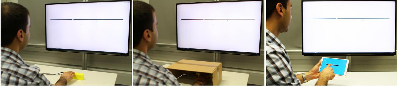
(a) Selecting a target value using the VMRS with VF. (b) Selecting a target value on the VMRS covered by a cardboard box (NVF). (c) Selecting a target value on the tablet with VF.
