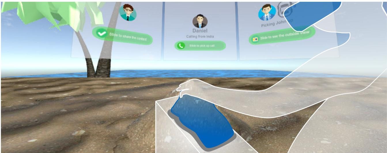
**Figure 1:** Our interactive armrest enables haptic and visual traces across real and virtual environments, which help users recall prior presence in everyday in-car VR.
