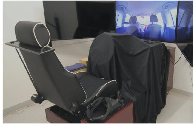
**Figure 5:** Our laboratory set-up consists of a driving simulator with a desktop PC, a display, and an Oculus Rift S headset (with a right-hand controller) connected to the desktop PC.
