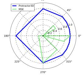
Figure 3. Polar plot of influence of rotation on the correct recognition rate. Protractor3D has a constant CRR under all rotations and thus is rotation-invariant, whereas MSE-only is highly susceptible to changes in the rotation of the input gestures, and in some cases falls back to zero recognized gestures.
